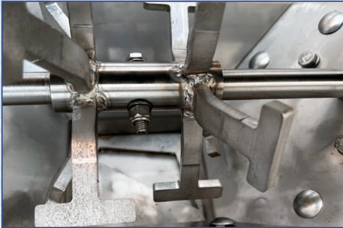
Electric crusher inside the hopper
