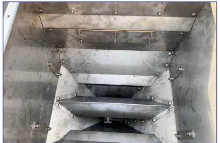
Internal metal protection hopper
