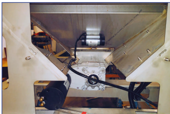
Electric engine 12 V 24 V with adapter for the auger rotation
