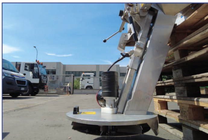
Electric engine 12 V 24 V for spreading disc rotation
