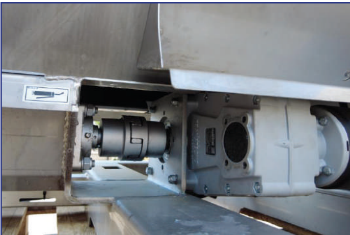
Adapter for screw conveyor with elastic/mechanic coupling
