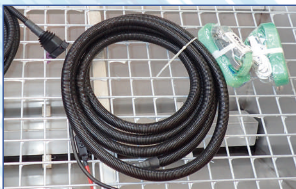
Battery cable connection kit and anchorage/fastening bands for fixing the salt spreader on the vehicle
