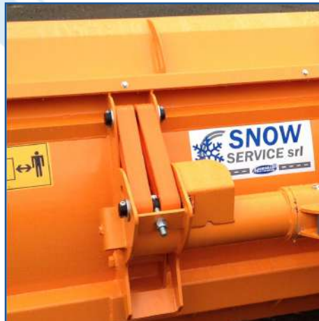
Polyurethane elastomers to prevent the snowplow tipping over
