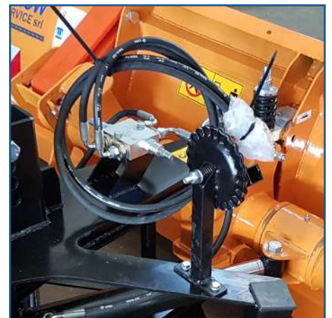
Anti-shock valves on the orientation cylinders
