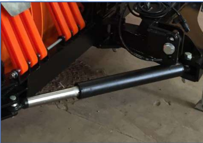
Hydraulic orientation with single-acting cylinders
