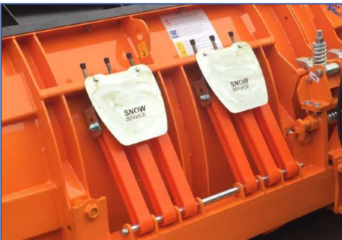
Polyurethane elastomers to prevent the snowplow from tipping over
