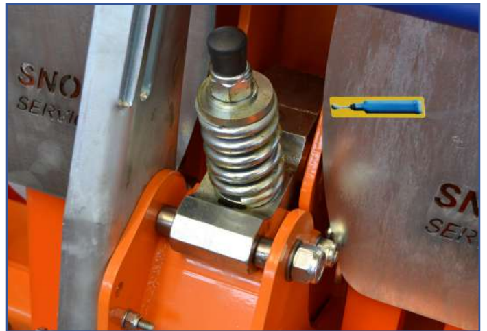
Retaining mechanical hooks to provide vibration protection
