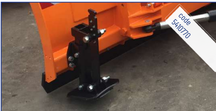
Pair of adjustable in height slides
