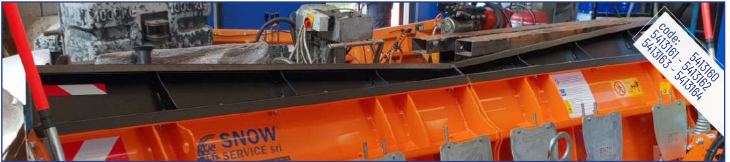
"V"- shaped steel upper extension
