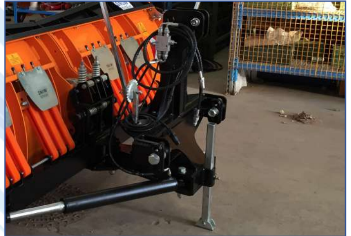
II and III category 3-point hitch lift system
