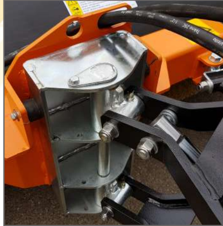
Central tilt mechanism for lateral oscillating movements
