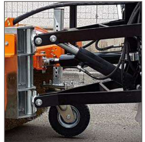
Double-effect lifting cylinder
