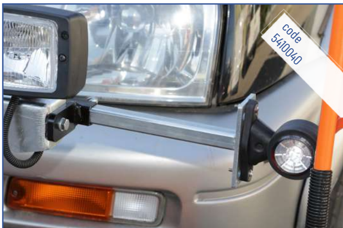
Led lights with extendable mobile support
