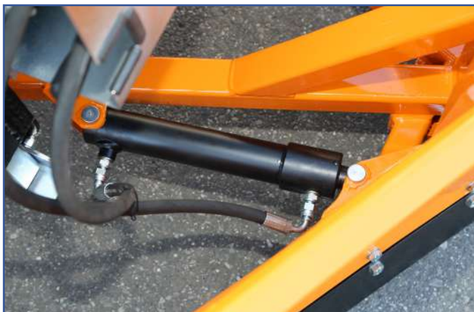
N. 2 double acting hydraulic cylinders to open/close the blade
