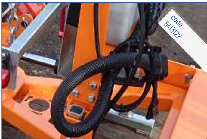
Bipolar electric cable for electrical connection to the vehicle battery
