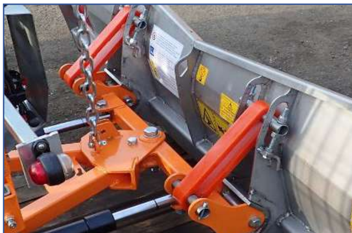
Shock-absorbing system through polyurethane elastomers
