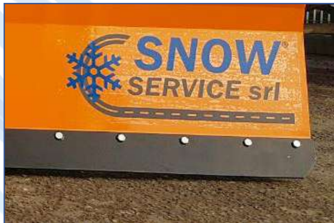
Steel wear resistant cutting edge
