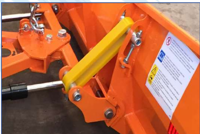
N. 2 single acting hydraulic cylinders to manage the blade orientation
