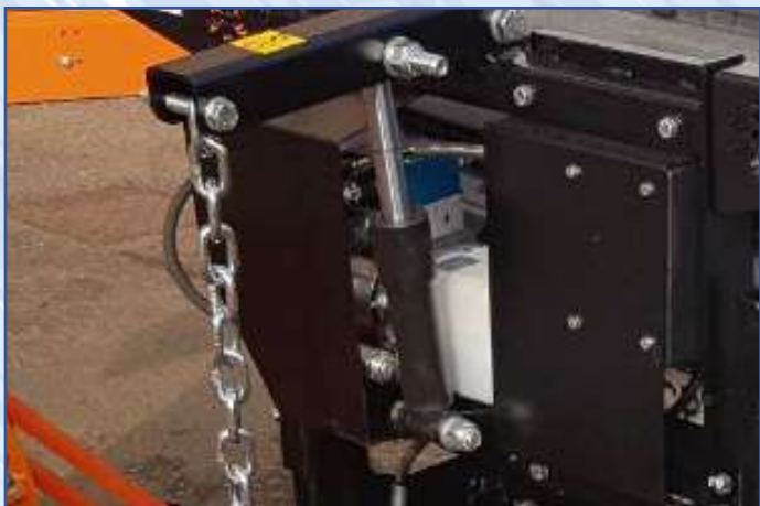
Single acting hydraulic lifting movement of the snowplow
