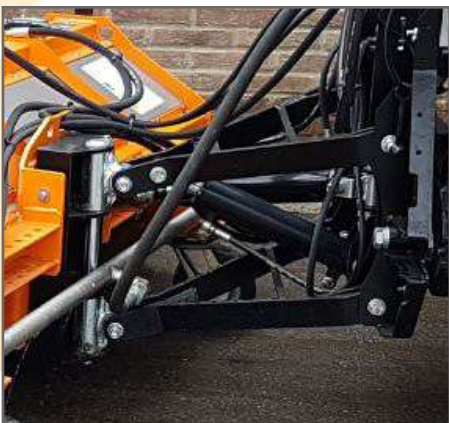
DIN type attachment plate with mechanical orientation
