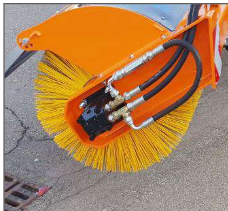
Brush with PPL rings \varnothing 600 mm
