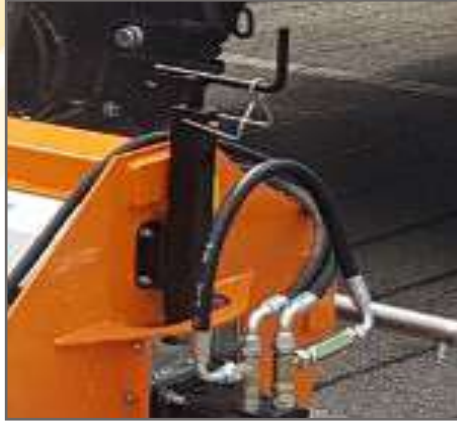
Mechanical adjustment of the roller height according to its wear
