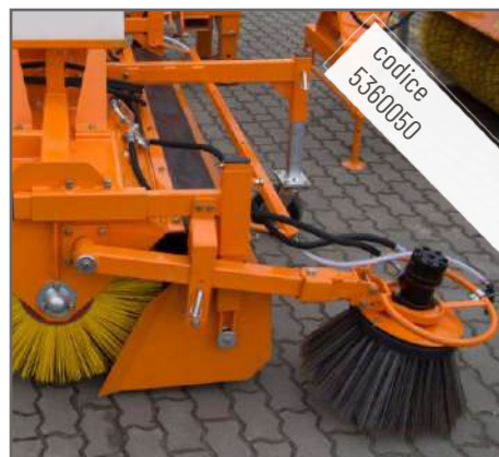
Hydraulic lateral brush with lifting cylinder
