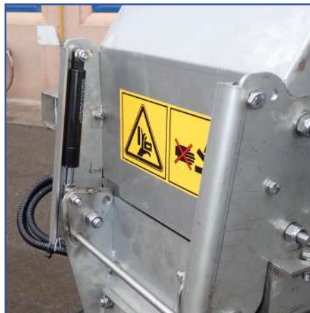
Gas spring for the lifting of the tower
