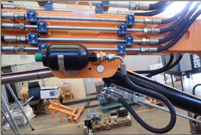
Nitrogen accumulator and block valve on the cylinders
