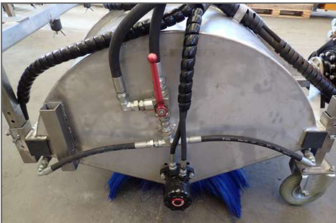
Hydraulic engine for brush swivelling
