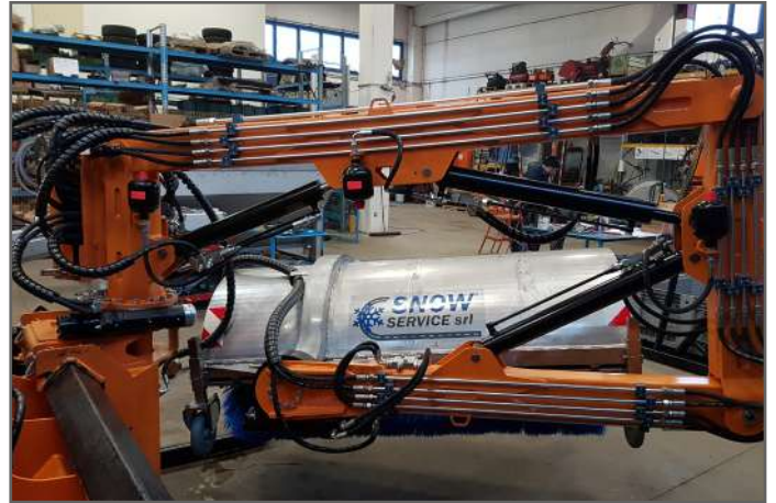
Nitrogen accumulators on the hydraulic cylinders to act as shock absorbers
