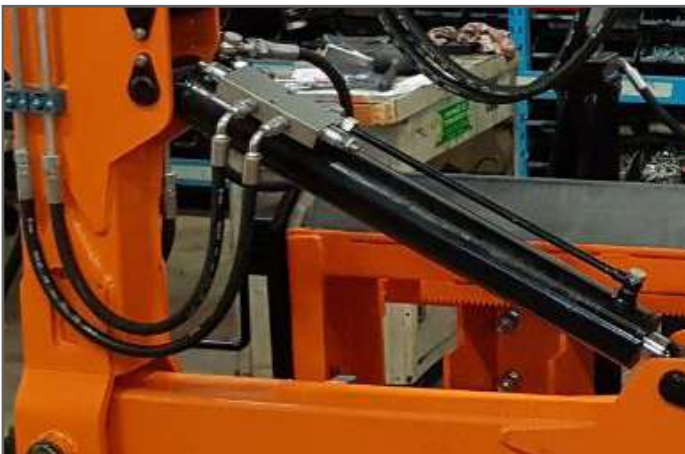
Hydraulic cylinders with block valves
