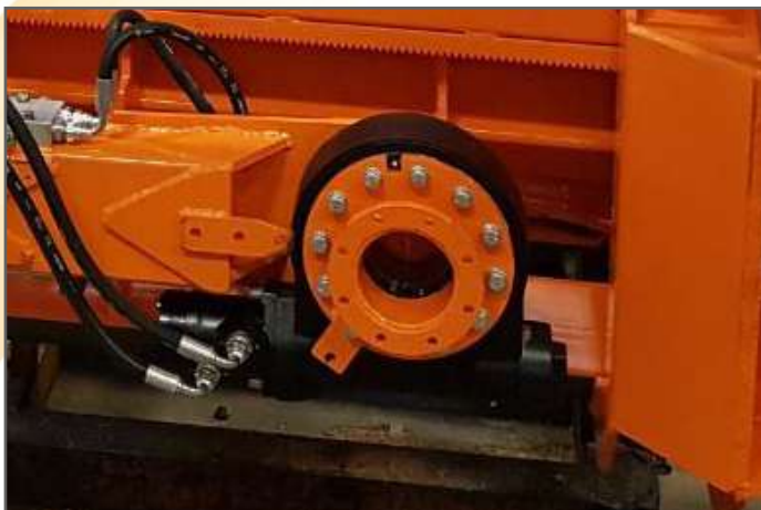
Hydraulic fifth wheel/circle frame for head rotation
