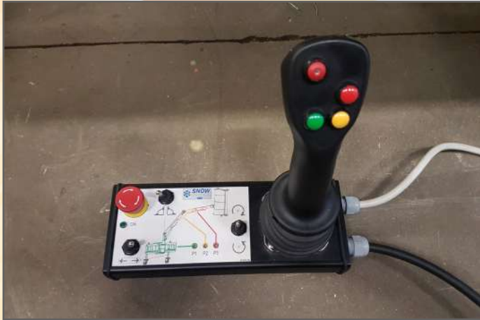
Electronic push-button panel with joystick
