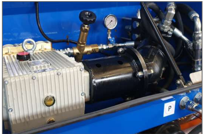
High-pressure hydraulically driven pump
