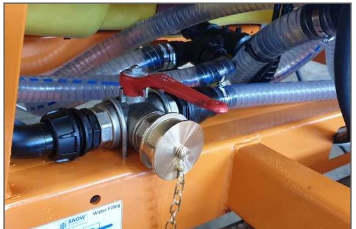
Manual valve with UNI-STORZ coupling for tank filling/empting processes
