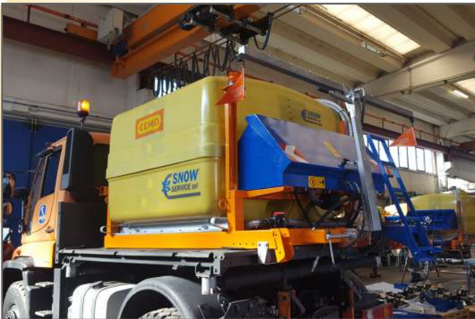
Parallelepiped-shaped fiberglass tank with internal breakwater walls (capacity available 2000 LT, 3000 LT, 4000 LT, 5000 LT)
