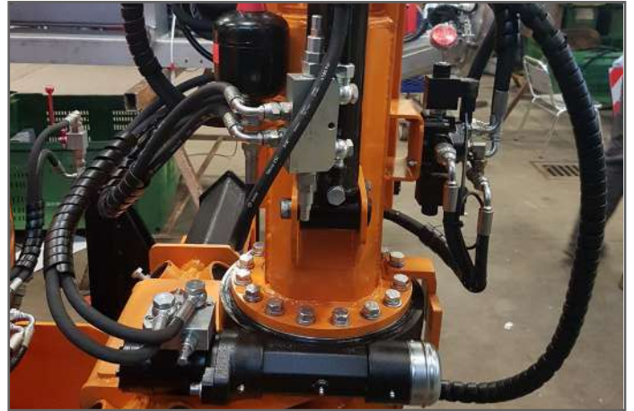
Hydraulic fifth wheel/circle frame for rotary movements
