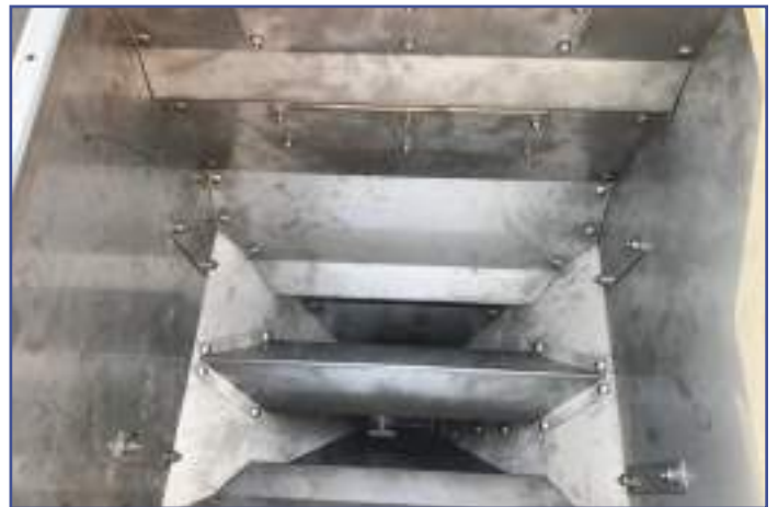
Internal metal protection hopper
