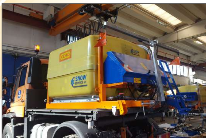
Cisterna in vetroresina forma parallelepipedica con pareti interne frangiflutti (cap. disp. 2000 LT, 3000 LT, 4000 LT, 5000 LT)
